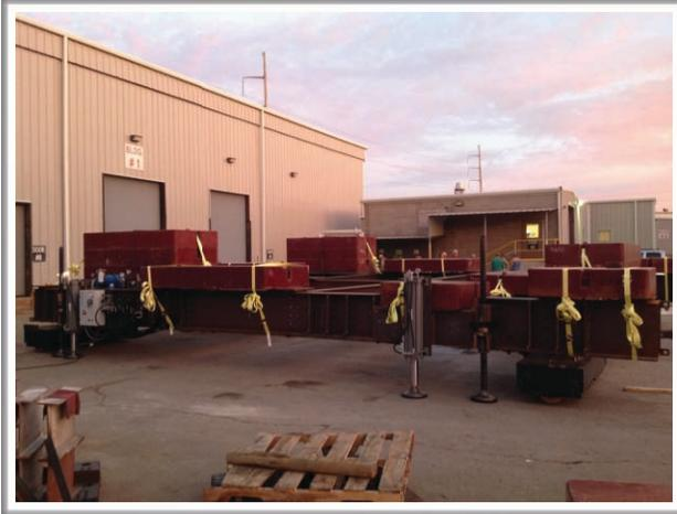
the spring would never bottom out. Clearly with a load of 125 tons, failure was not an option. As you can see from the photo to the left, loads of similar capacity were simulated using metal weights placed on steel girders.
