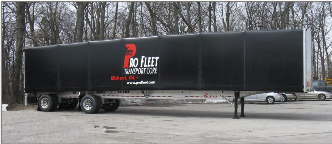
Roll Tite manufactures retractable tarpaulin systems that turn a 53-foot flat bed trailer into a rig that can carry a full cargo load but with greater flexibility. The tarpaulin can be completely customized and is mounted on a number of bows attached to a wheel/rail system that allows it to retract.
