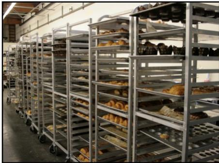
If you've ever been in a bakery plant, you know that it's an incredibly demanding environment. Dough, and the racks on which it is baked, go from room temperature to almost 500 degrees Fahrenheit then back to room temperature. In addition, those racks are used to transport the finished baked goods through warehouses, into trucks, to customer locations and then come to the plant to start the cycle all over again.
